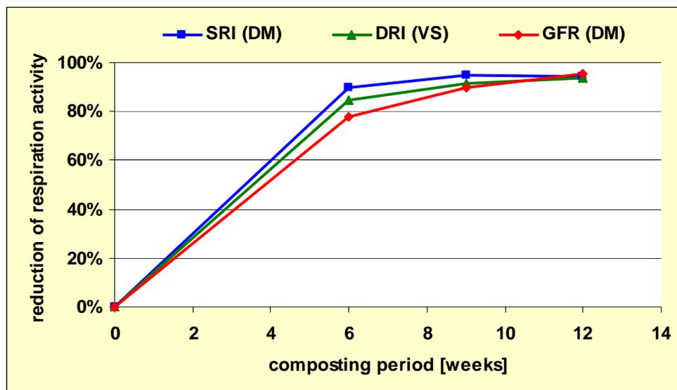
**Figure 3. Reduction different measure of biodegradability (using SRI, BOD<sub>4</sub>) during the composting of MSW using New Earth Composting Technology.**
