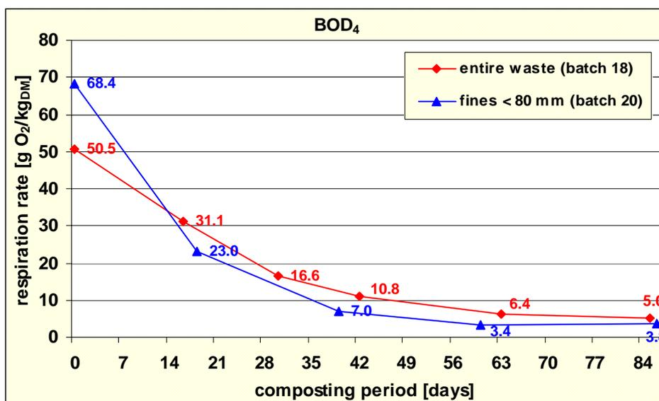
Figure 2: **Change in respiration rate (using SRI, BOD<sub>4</sub>) during the composting of MSW using New Earth Composting Technology.**
