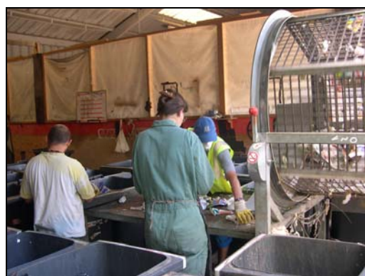
Figure 2: Collected waste ready for sorting, and waste passing through the trommel screen for sorting into categories.
